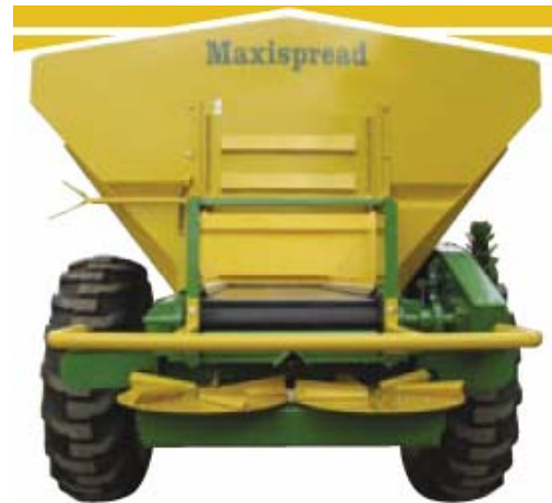
Photo 2. Horizontal flat spinners are also effective in spreading over a wide area. Landaco Maxispread. www.landaco.com.au
