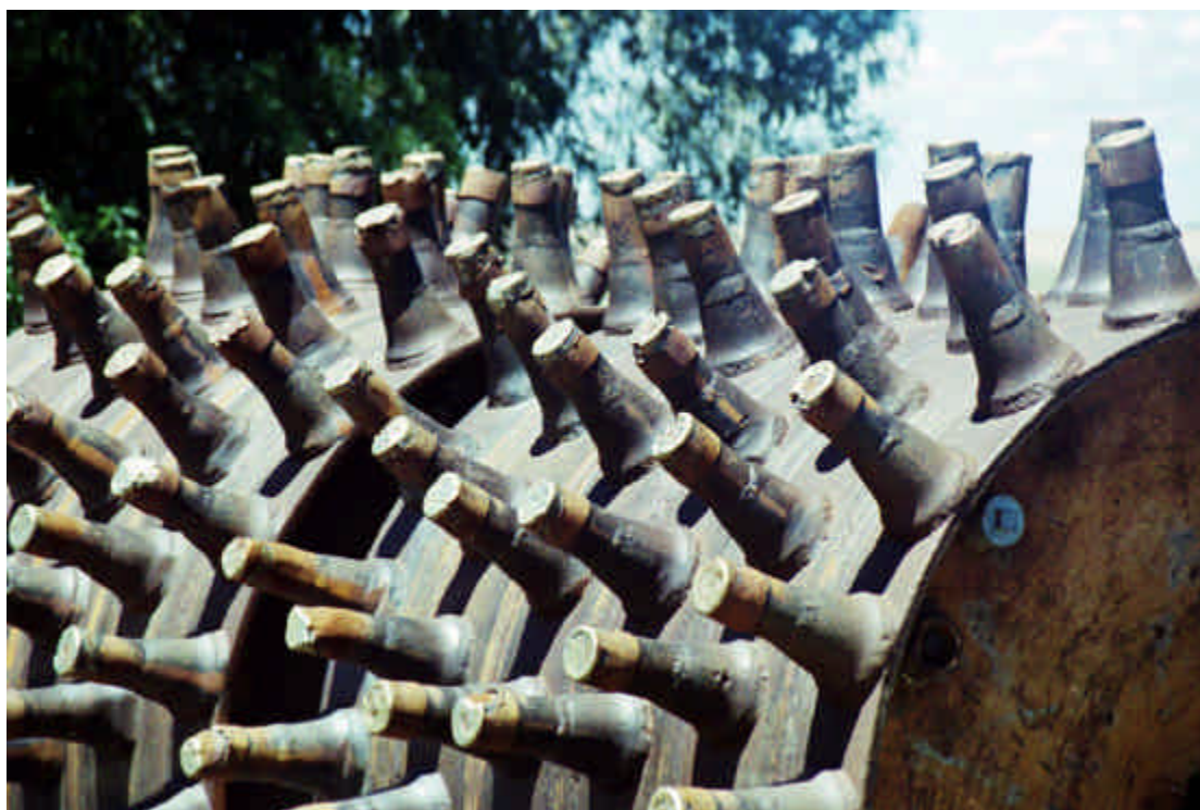
PHOTOGRAPH 5-2 – CLOSE UP OF SHEEPSFOOT ROLLER
