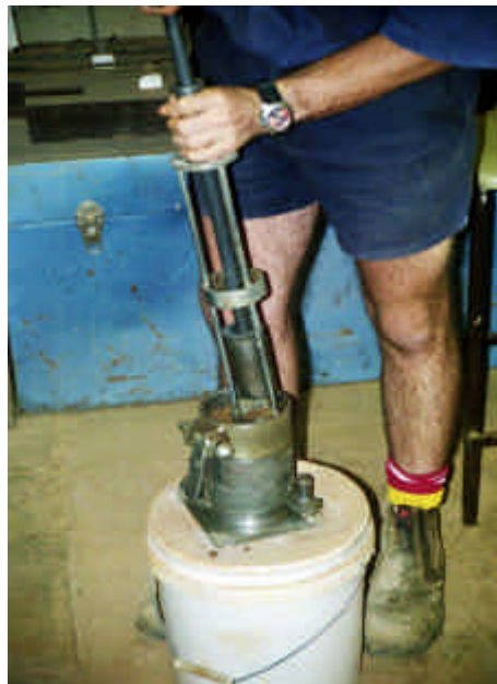
PHOTOGRAPH E-4 – UNDERTAKING COMPACTION TEST IN LABORATORY
