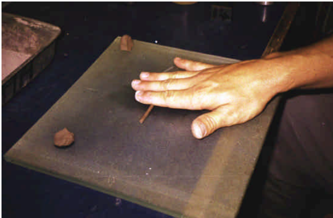
PHOTOGRAPH E-1 – ROLLING CLAY TO DETERMINE PLASTIC LIMIT
