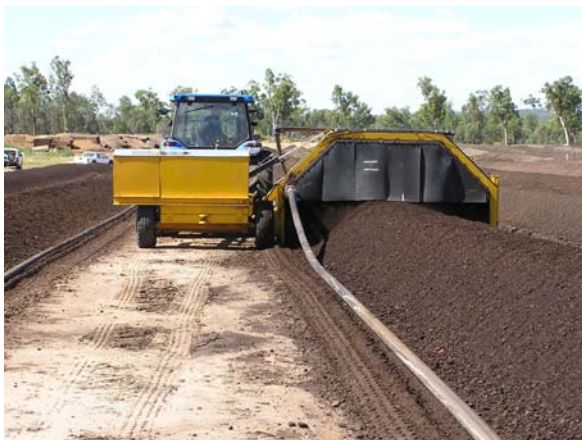
Photo 1. Tractor drawn windrow turner with water application during turning.
