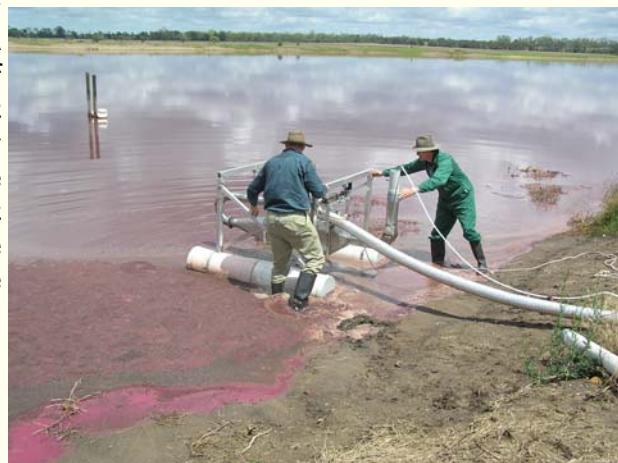
QDPI staff floating odour sampling equipment out into a feedlot holding pond.
